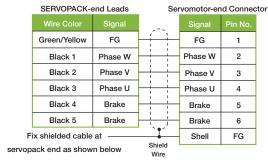
Note: No polarity for connection to a holding brake.
