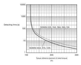
Note: Overload characteristics shown above do not guarantee continuous duty of 100% or more output. Use a servomotor with effective torque within the continuous duty zone of Torque-Speed Characteristics.
